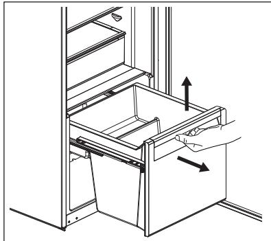
2. Push the rails inside the cabinet to avoid damage to the appliance when closing the door.
